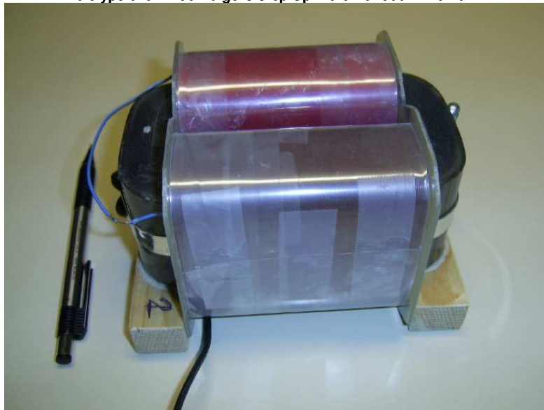
Prototype of a 1:150 "rutgerS'Step Up Trafo" for 300 Hz to 20 kHz
