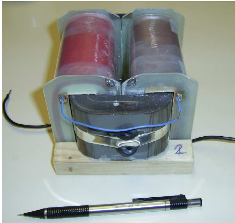
Prototype of a 1:150 "rutgerS'Step Up Trafo" for 300 Hz to 20 kHz
