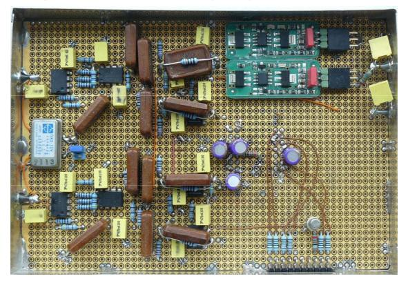
To investigate if the absolute fase 'is right', the audio output should go negative if the DSD-signal in question is chortcuircuited. By the way: R3 and R13 are not implemented!
