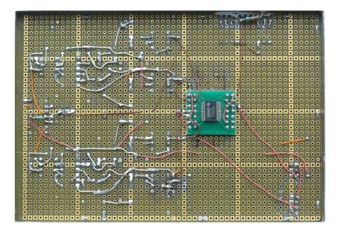
The completed board with two TentLabs stabilisers (3 & 5 volt) for the PCM1792 could look like:
