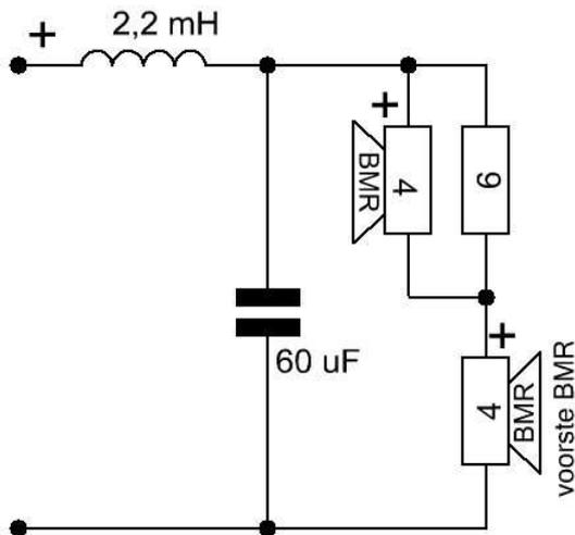
The 'voorste BMR' means: the BMR in the front of the baffle. The other one is at the rear side, which has been shunted by a resistor of 6  $\Omega$ . The effect is that the front speaker radiates about 2.5 dB more than the rear speaker which effects the total radiation pattern to give a better sound image.
