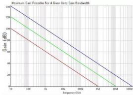
You can see that the compensated graph in blue has a very orderly slope of 6 dB/octave, and a phase shift of around 90° over most of the frequency range. This is the characteristic of a single pole roll off. It is created by a single capacitor purposefully placed inside of the device to roll off and reduce the gain to zero before the poles from the parasitic capacitors internal to the op amp come into play.
