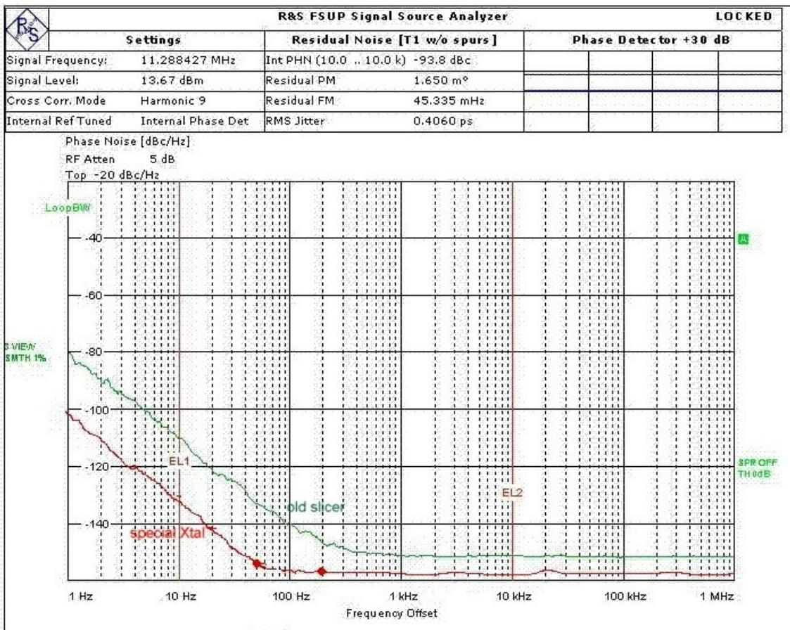
Two things should be clear: The noise floor of my oscillator is much lower than that of the oscillator of Mori. More over: **the noise does not enhance at frequencies nearer than 10 Hz from the carrier!!** Mind that we talk about two the same circuit diagrams!
